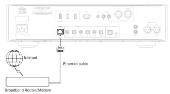
Connect a network cable (Category 5/5E straight through Ethernet cable) between the 851N and your router.
