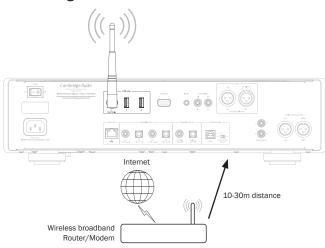
Connect the supplied wireless antenna to the correct USB input on the rear of 851N – it will need to be in range of your wireless router.
